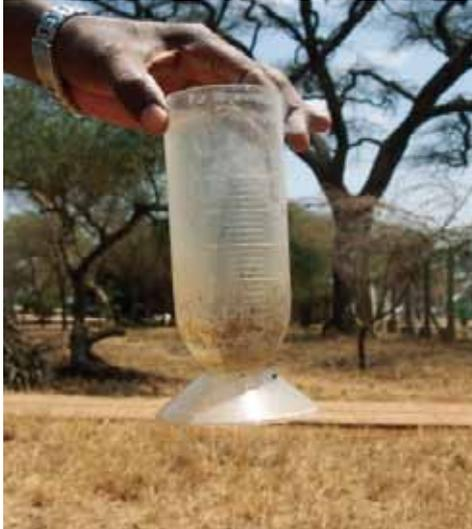
Figure3. Inside cup of rain gauge
